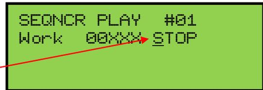
Press the **MEMORY** button to stop playback. The counter will reset to zero (0) and the instrument will stop playing indicating playback has stopped.
