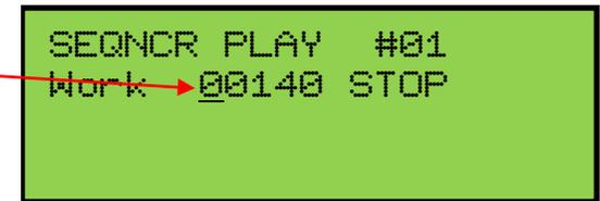
Press the **CURSOR** button to position the cursor on the Transport Control Function.
