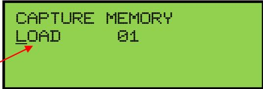
Select a Capture File Number. Press the **CURSOR** button to position the cursor on the Capture File Number value.
