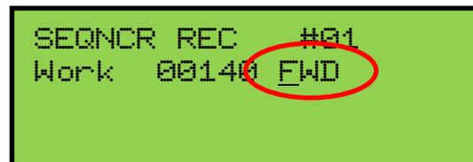
Press the **MEMORY** button to resume recording. The counter will start counting from the current counter value to indicate that recording has resumed.
