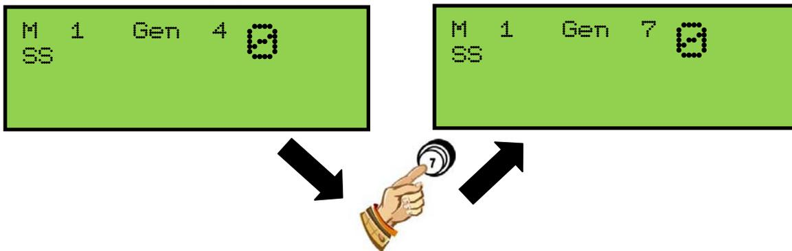
The capture memory level may also be changed at any time while within the SIMPLE STEPPER mode. To change the capture memory level, press the **CURSOR** button to position the cursor on capture memory level value. Then, turn the **ROTARY DIAL** to select a different capture memory level (*see Section A-3*).
