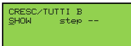
To view the stops/drawknobs registered on the second (B) TUTTI I or TUTTI II, press either TUTTI. This will cause all associated stops/drawknobs programmed on the selected TUTTI to turn on.
