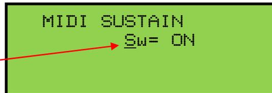
To turn the MIDI Sustain function on/off on the selected manual, press the **CURSOR** button to position the cursor on the MIDI Sustain value.
