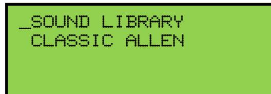
To change to a different voicing specification, press the **CURSOR** button on the GeniSys™ Controller and position the cursor on the voicing specification name. Turn the **ROTARY DIAL** to select a different voicing specification.
