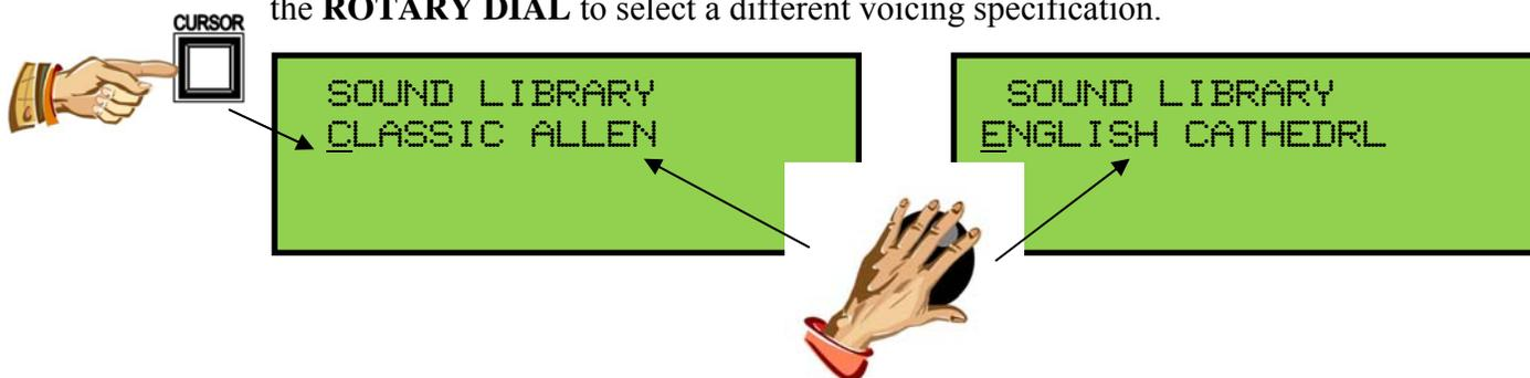
When the desired voicing specification is displayed, press and hold the **SET** piston. Then, while holding **SET**, press the **MEMORY** button on the GeniSys™ Controller. Release both.
