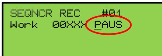
To "pause" the Sequencer during the recording, press the **MEMORY** button. The counter will stop counting indicating the recording has stopped. The Transport Control Function will revert back to "FWD" indicating the recording may be resumed at the current counter value.
