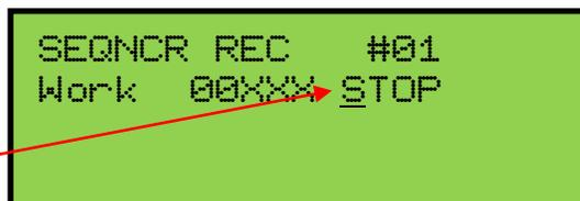
Finally, press the **MEMORY** button. This will stop the recording and automatically set the Sequencer into playback mode.
