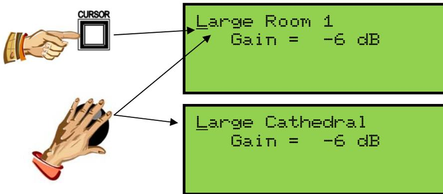
**Note:** The change will not be immediate. You must wait 3 seconds for the newly selected Acoustic Portrait pallet to load. The display will indicate that the newly selected pallet is loading:
