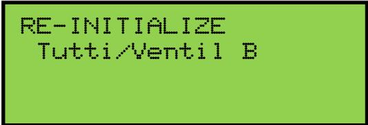
The Piston Configuration re-initialization includes all the Configure Piston settings. The MIDI Settings re-initialization includes all MIDI program change mapping. The Capture Memory re-initialization will reset the last available capture memory to factory default registrations (*if applicable*).
