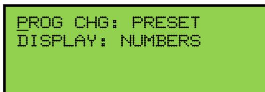
Press the **CURSOR** button until the cursor is positioned on the Program Change mode value.
