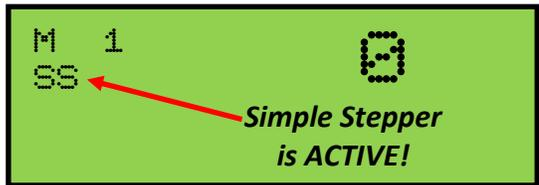
To start SIMPLE STEPPER, select a capture memory level (*see Section A-3*) and then press General piston #1. The registration associated with the selected capture memory level and General piston #1 will register on the stops and the display will indicate that General #1 has been pressed. This will also set the SIMPLE STEPPER’s starting step position.
