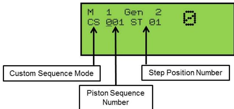
To select a piston sequence number, press the **CURSOR** button to position the cursor on the piston sequence number.
