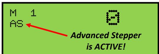
To start ADVANCED STEPPER, select a capture memory level (*see Section A-3*) and then press General piston #1. The registration associated with the selected capture memory level and General piston #1 will register on the stops and the display will indicate that General #1 has been pressed. This will also set the SIMPLE STEPPER’s starting step position.
