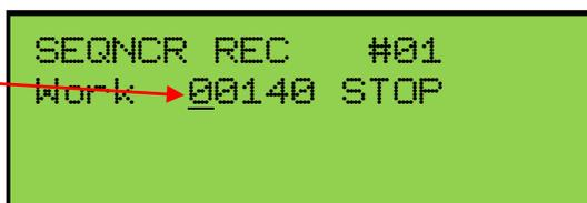
Press the **CURSOR** button to position the cursor on the Transport Control Function.
