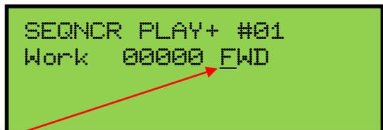
Press the **MEMORY** button to begin playback. The counter will start counting to indicate that playback has started.
