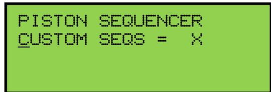
To use the CUSTOM SEQUENCER mode, return to the *Main Window* function. Press and hold the **SET** piston. Then, while holding **SET**, press the **CANCEL**.
