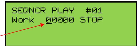
Turn the **ROTARY DIAL** to select a different counter value. Turning the Rotary Dial clockwise will increase the counter number while turning the Rotary Dial counter-clockwise will decrease the counter number.
