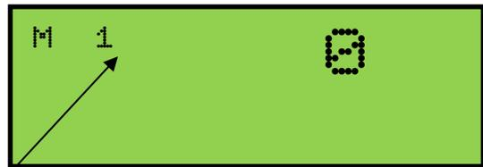
desired capture memory is selected, press and hold the **MEMORY** button in the GeniSys™ Controller. Then, while pressing **MEMORY**, enter the same three-digit code that was used to lock this memory (See Section A-5). Release the **MEMORY** button. If the correct
