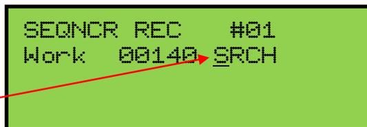
The “SRCH” function scans the MIDI song from the beginning of the MIDI song file up to the current counter position for any messages pertaining to the organ's stop registrations and expression data. The Sequencer will setup the organ with the scanned settings so it is prepared to resume recording the MIDI song file from the current selected counter position.
