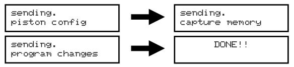
The 'dot' behind the word 'SENDING' on line one of the display will move as the data is transmitted.
