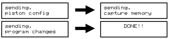
The 'dot' behind the word 'SENDING' on line one of the display will move as the data is transmitted.
