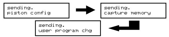
The 'dot' behind the word 'SENDING' on line one of the display will move as data is transmitted.
