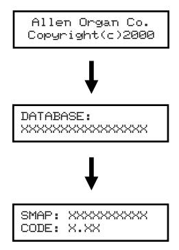
**Note:** The LCD will display the current stopmap level (SMAP) and operating software base code level (CODE) currently installed in the organ.
