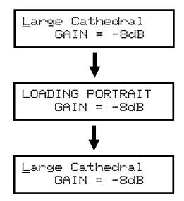
If the organ is equipped with a Quad Suite<sup>™</sup>/Stoplist Library<sup>™</sup> Display Window, it will also flash while the new pallet is loading. Once the newly selected pallet is loaded the display will change back to the Acoustic Portrait<sup>™</sup> pallet name and the Quad Suite<sup>™</sup>/Stoplist Library<sup>™</sup> Display Window will stop flashing.
