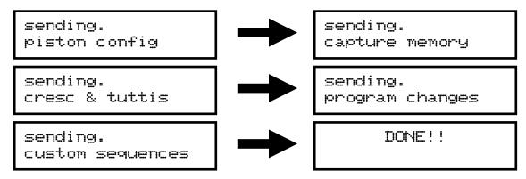
The 'dot' behind the word 'SENDING' on line one of the display will move as the data is transmitted to the sequencer.
